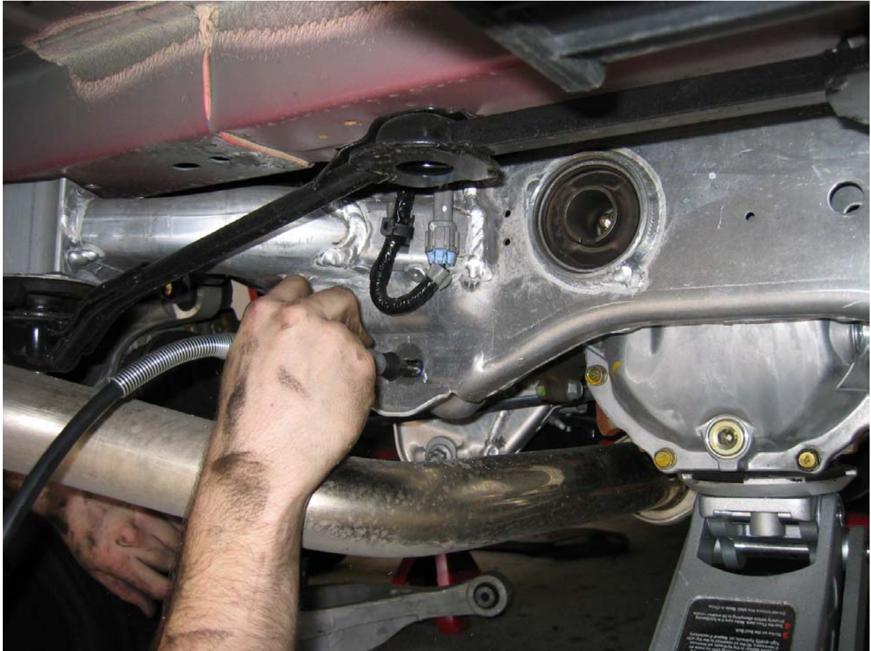
Picture during grinding. You are only elongating the slot.
